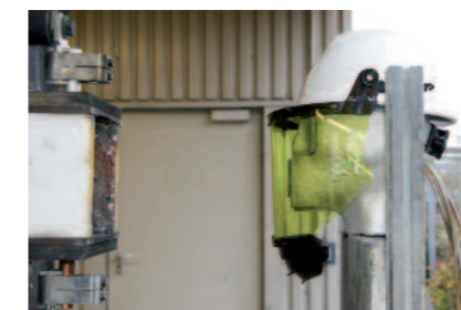
MSA arc flash set before "arc-in-the-box testing" 7 kA
