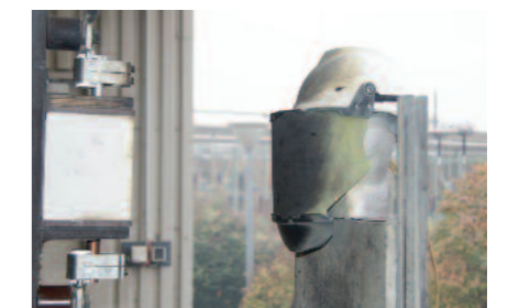
GS-ET-29 class 2-7 kA certification passed. Head and face combination protects the wearer
